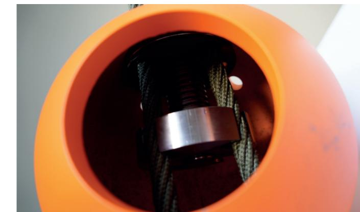
**The patented system has interlocking gears that allow more than one tensioning system within the spherical connector. It also allows the stretching process to be performed from outside so it provides an easier assembly and stops the lid from being removed constantly to repair as well as prevent possible breakages.**
