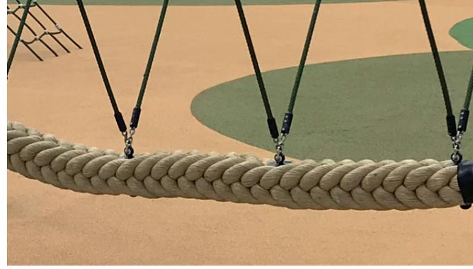
**The rope used as a swaying station in the middle of the product should be made of 8 braids, forming in a square form, with a diameter of 140 mm and a minimum length of 550 cm, through which Ø10 mm steel winding rope passes inside.**
