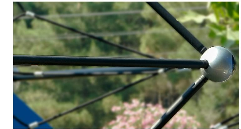
**Metal parts are comprised of ST 37 Steel with a 3-step metal finish. Sandblasting and solvent-free zinc primer coating and electrostatic powder paint application is inherently corrosion resistant under extreme weather conditions and UV.**
