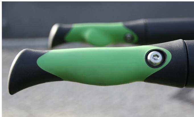
**Ergonomic handles are made using plastic co-injection with an elastomer cover. 55-shore elastomer provides a soft feel with UV resistance. 2-layer design has good grip and prevent sweating, making it easy for everyone to use them comfortably.**
